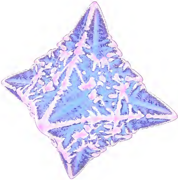
Fig. 19. A 3D dendrite visualized using glyphs and semi-transparent colors. This image was generated from the same data as in Fig. 17. In this image the output from the simulator has been mirrored along all three axes giving a symmetric six-pointed star structure. The image in Fig. 17, due to memory limitations in computing the iso-surface, was mirrored only along the x and y axes.
